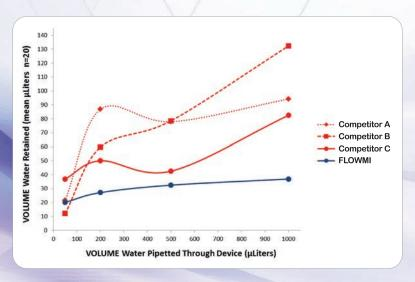
FLOWMI™ and three competing strainers were examined at four pipetted volumes (50, 200, 500, and 1000 µl). The Volume of Water Retained (µl) by each strainer, at each pipetted volume, is represented by the mean difference in weight before and after pipetting water through the strainer. (n=20 per pipetted volume; each trial using a new strainer).
