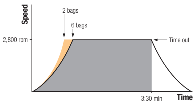
Figure 1. In a typical first centrifugation step, a two-bag rotor load attains set speed faster than a six-bag load. Since both loads will time out at the set time of 3:30 minutes, different g-forces are achieved during the run. By using the ACE integrator function, the time for 2 bags would be changed to 3:00 minutes to obtain the same overall g-force for both loads. With an ACE value and speed set at the start of a run, times were adjusted to achieve the same overall g-force regardless of the rotor load.
